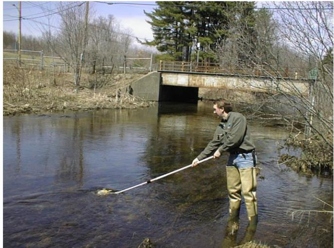
**CAUTION:** Do not extend the pole too far when sampling high velocity streams. You’d be surprised at how much force there can be on the pole. To avoid damaging (bending) the pole, it is recommended that you leave at least 1-foot un-extended.
